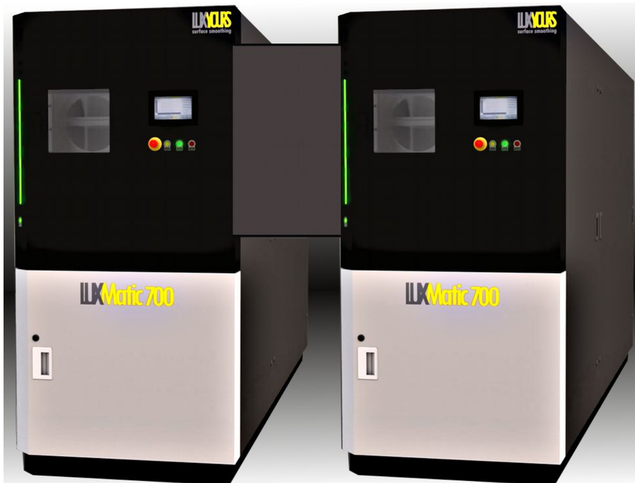
Two LUXMatic 700 coupled with a tunnel for smoothing of 2m long parts.
